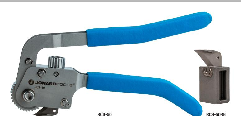
Designed to open the toughest heavy-duty cable jackets, the RCS-50 is perfect for performing lateral and longitudinal cuts on submariner cables, large fiber ducts, or large count telephone cables at least 1 1/2" (3.81 cm) in diameter. This ratcheting cable slitter also features the following:
